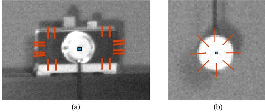
Fig. 3. Measurement models. (a) 16 measurement lines are used to identify and track the cart. (b) 8 radially symmetric measurement lines are used for the pendulum. In both cases the sample that gave rise to the measurement lines is depicted as blue square.
