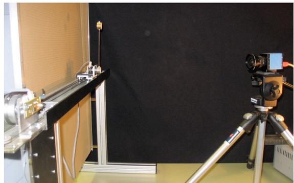
Fig. 4. Inverted pendulum prototype. The cart, pendulum, and parts of the driving DC motor are shown on the left. A firewire camera is used to provide visual feedback for the control algorithm. In this prototype both vision-based tracking and commercially available Hall sensors can be used to measure the state of the pendulum.
