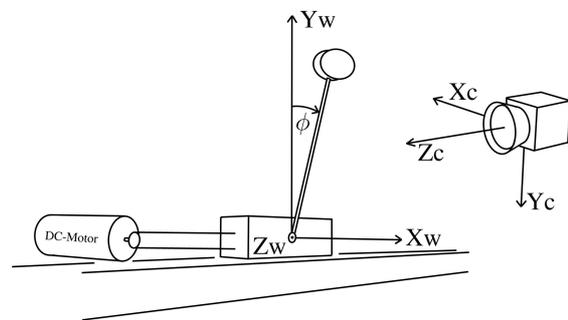
Fig. 1. Sketch of inverted pendulum. The aim of the experiment is to balance the pendulum in its upright position ( $\phi = 0^\circ$ ) by means of providing control signals to the DC motor which in turn drives the supporting cart.
