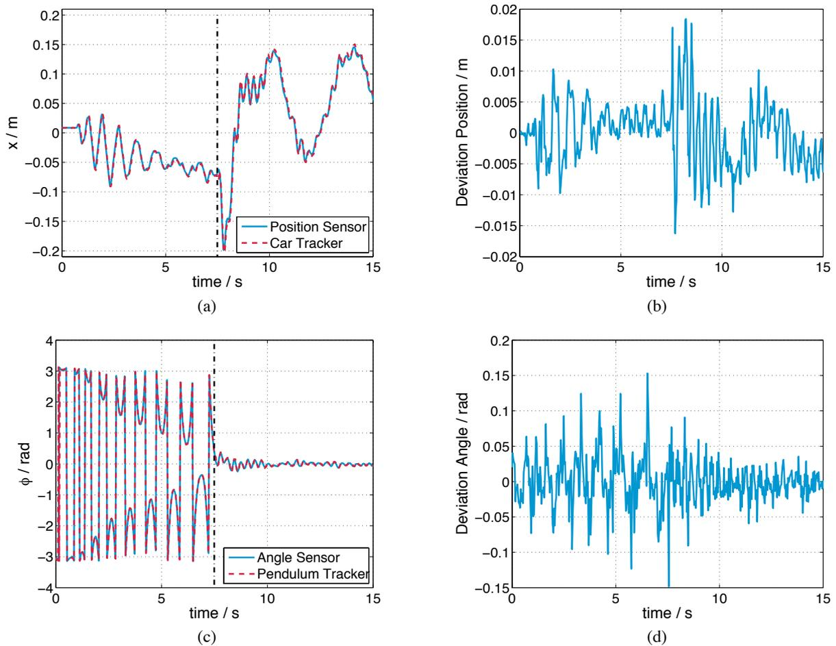
Fig. 5. Measurement results of the vision-based tracking algorithm. (a) Position of the cart measured by the Hall sensor and the particle filter PF1. The deviations of the PF1 result w.r.t. the Hall sensor are shown in (b). (c) Orientation angle of the pendulum as observed by the Hall sensor and PF2. Again, deviations are shown in (d). The vertical lines at  $t \approx 7.5$  s in (a) and (c) denote the point where the application switches between swinging-up and balancing of the pendulum.
