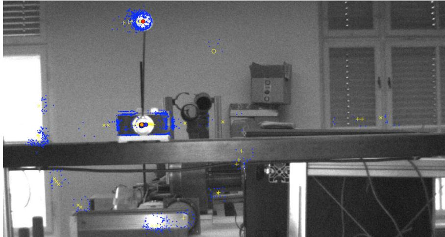
Fig. 6. Different types of samples (yellow) and the resultant contour detections (blue) superimposed to a camera frame: Standard resampling (+), importance sampling (x), and initialisations (o). Samples used by the cart tracker are distributed horizontally along the cart track while samples used by the pendulum are distributed along the ellipse centred at the cart representing possible pendulum locations.
