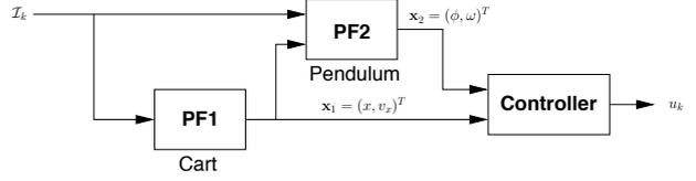
Fig. 2. Block diagram of the inverted pendulum control algorithm. Two Particle Filter trackers are used to estimate the cart position and velocity (PF1) and the pendulum angle and angular velocity (PF2) given the most recent image  $\mathcal{I}_k$ . Based on these inputs the controller provides the control signal  $u_k$  for the DC motor.
